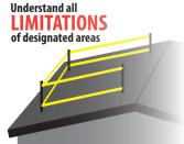
A designated area must be delineated by a warning line. The line has to be constructed out of rope, wire, tape, or chain that is as close to the work area as possible. The warning line must:
